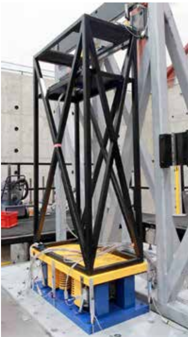
Ruskin Dam isolation system tested at the University of Nevada, Reno.
