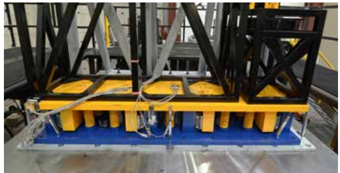
3D Isolation System was tested at UNR.
