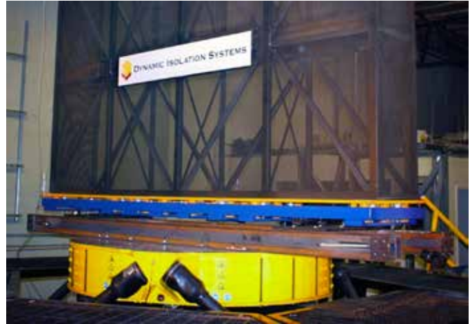
3D shake table testing of DIS' 3D isolation system at Dynamic Certification Laboratories.
