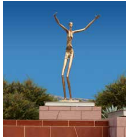
These 20 foot tall bronze statues in a California park are isolated on DIS platforms capable of moving \pm 30'' in an earthquake.
