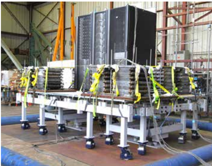
3D shake table testing of DIS' floor isolation system at the University of California, Berkeley.
