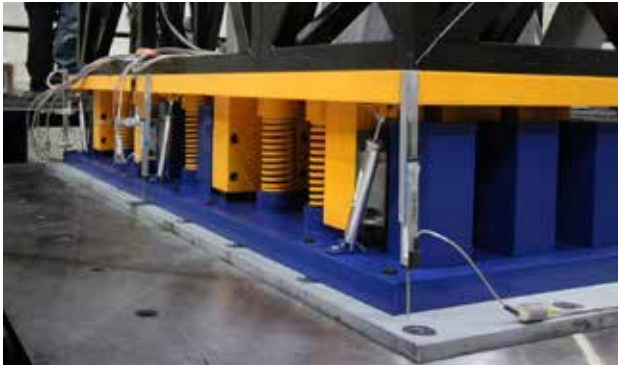
Shake table testing of DIS' vertical isolation system at the University of Nevada, Reno.
